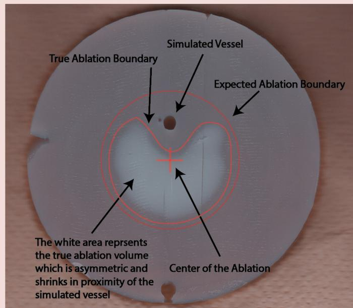
**Figure 2** - Slice of a cylinder made of tissue mimicking gels into which an ablation has been performed. The gel is dyed with a substance that turns white under temperature and which indicates the volume of the tissues that would be killed in a person.
