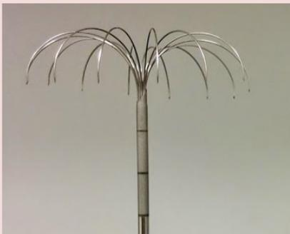
**Figure 1** - Typical electrode for Radio Frequency Ablation: the electrode is formed by a shaft (diameter 3mm) and by an umbrella of tines (diameter of the umbrella 5cm) which can be retracted inside the cannula for insertion into the tumor location, and later expanded to encompass the tumor tissues.
